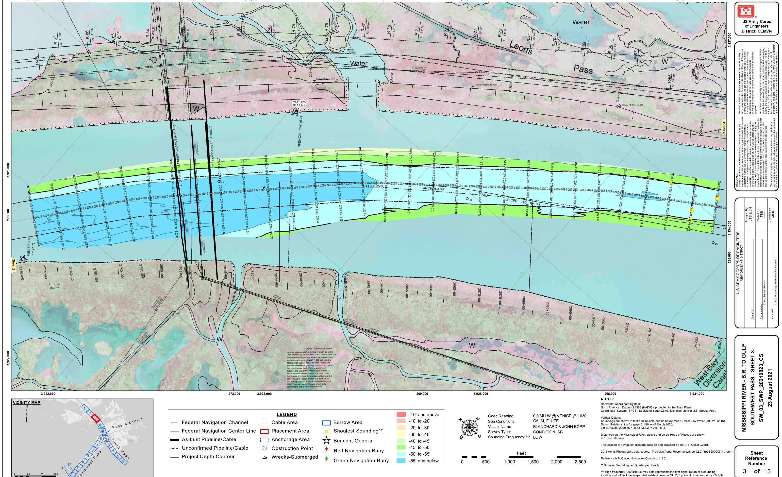
survey data normally penetrates through this "fluff" layer to depict elevations of consoldiated bottom material. Low frequency accuracies may vary depending on channel conditions and fathometer
